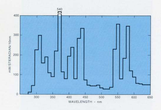
ADVANCED RADIATION CORPORATIONS' 200 Watt A.C.-D.C. Mercury Short Arc Lamp is designed and manufactured to produce high intensity ultraviolet radiation for exposing photoresist materials. Operating with either A.C. or D.C. power the lamps exhibit stable performance and long reliable life. Other applications include photochemistry, micro-film enlargement and optical instrumentation.
