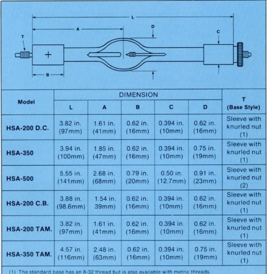
Mercury lamps operate with an internal pressure that approaches 40 atmospheres and the erythemal flux is extremely high. A shielded enclosure should therefore be used for protection. When cold, the lamp is at a reduced pressure and is safe to handle.
