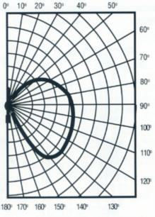
The shadow effect of the electrodes and the construction of the lamp limits the output to about 10 steradians as is illustrated in the polar distribution.
